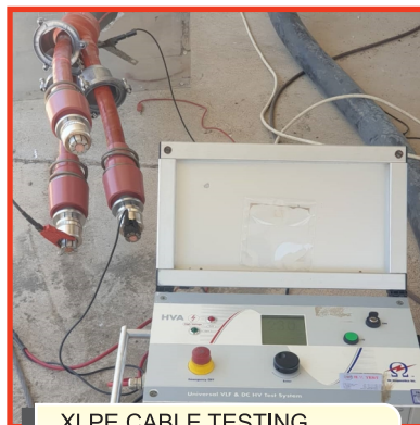
XLPE CABLE TESTING USING A VLF MACHINE
